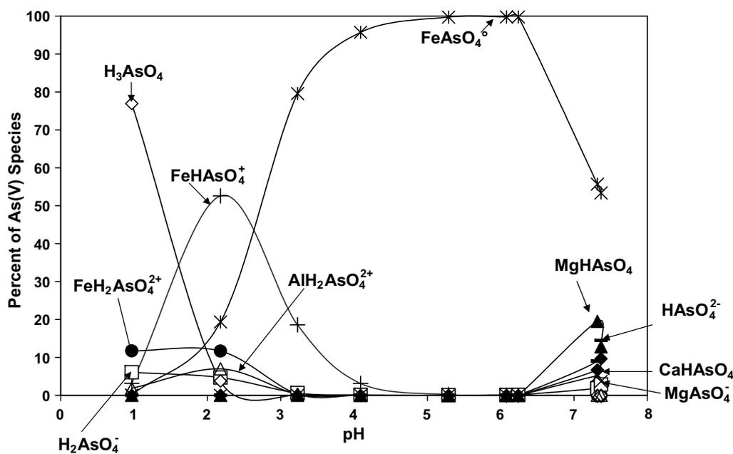
Fig. 9. Percent distribution of As(V) aqueous complexes in batch experiments during neutralization of Raffinate 2 with slaked lime. The figure is computed with PHREEQC, based on the chemical analytical data in Table 1. The Fe and As concentrations used in the calculations are the Fe(III) and As(V) chemical analyses from Table 1.
