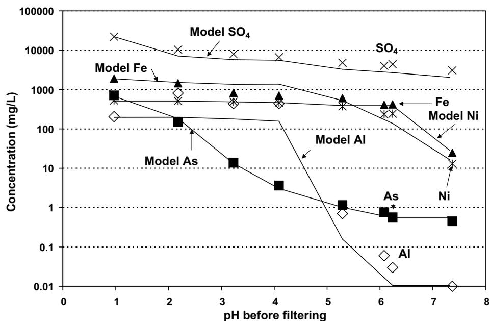
Fig. 13. Model fits (lines) of the concentration data (points) measured during neutralization of raffinate with slaked lime. Modeling assumptions and results are summarized in Table 4. Symbols:  $\text{SO}_4 = \text{X}$ , Fe = triangle, As = square, Ni = lined X, Al = diamond.
