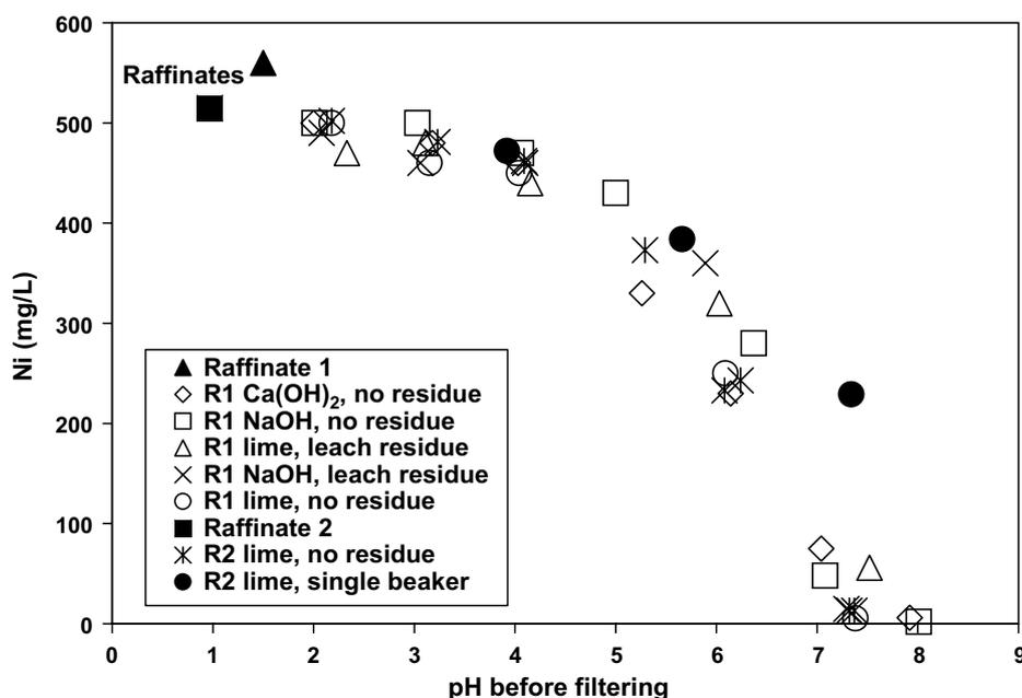
Fig. 5. Nickel concentrations as a function of pH in all of the raffinate neutralization experiments. Raffinate 1 (R1) and Raffinate 2 (R2) are shown as a solid triangle and solid square, respectively. Experiments were performed with and without mineral leach residues, and used lime (CaO), slaked lime (Ca(OH)<sub>2</sub>), or NaOH as added bases.
