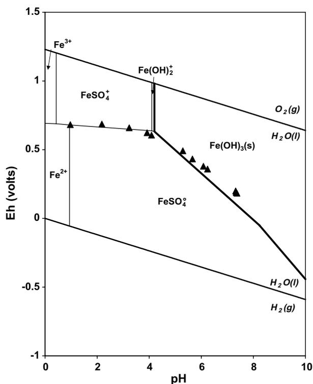
Fig. 10. Theoretical Eh–pH diagram for the system Fe–O–H–S–CO<sub>2</sub> neglecting sulfide aqueous species and solids. Triangles denote Eh values computed with PHREEQC from measured Fe(III) and Fe(II) concentrations. The Fe(OH)<sub>3</sub>(s)/solution boundary is drawn (in bold) for a dissolved Fe concentration of  $10^{-5} \text{ mol L}^{-1}$ . The solution contains  $\text{SO}_4^{2-} = 0.1 \text{ mol L}^{-1}$  and  $\text{HCO}_3^- = 10^{-2.7} \text{ mol L}^{-1}$ .
