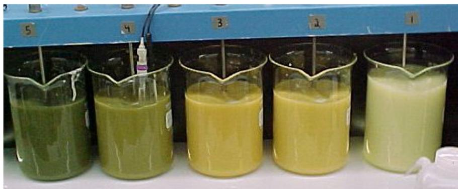
Fig. 2. Experimental setup in the batch tests at near final pH values for Raffinate 1 neutralized with slaked lime. The pH values in beakers 1–5 from right to left were 2.18, 3.15, 4.04, 6.09 and 7.38.
