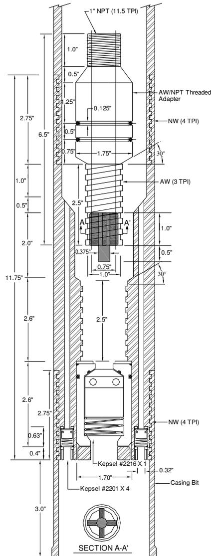
Figure 3. Details of footvalve
