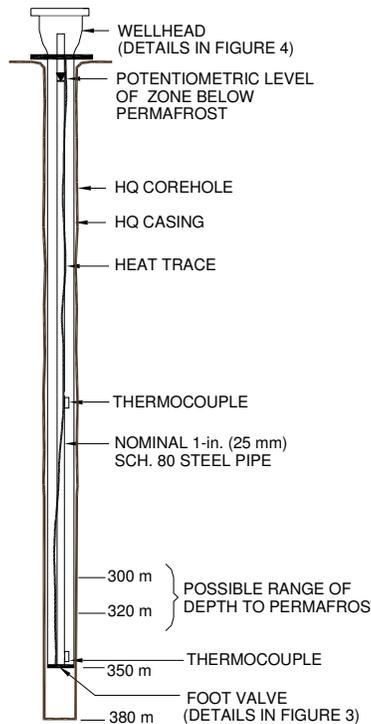
Figure 2. Schematic diagram of sub-permafrost monitoring well
