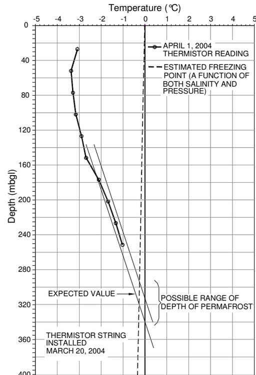
Figure 1. Thermistor data indicating depth of permafrost
