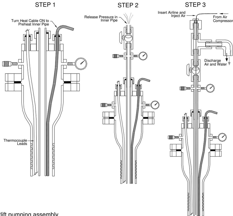
Figure 5. Airlift pumping assembly
