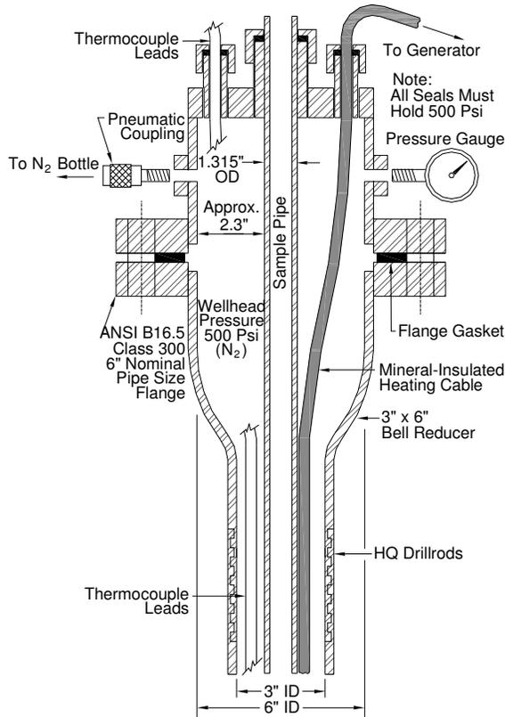
Figure 4. Details of wellhead
