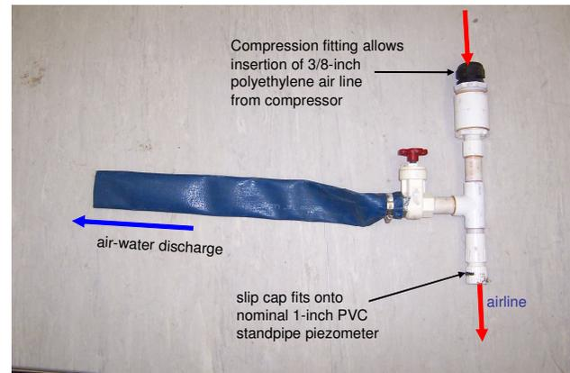
Figure 1. Simple device for airlift pumping groundwater samples from small diameter piezometers
