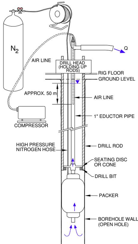
Figure 4. Small-educator method for airlift testing low permeability materials
