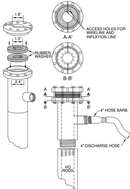
Figure 3. HQ wellhead assembly for packer-isolated airlift testing and sampling
