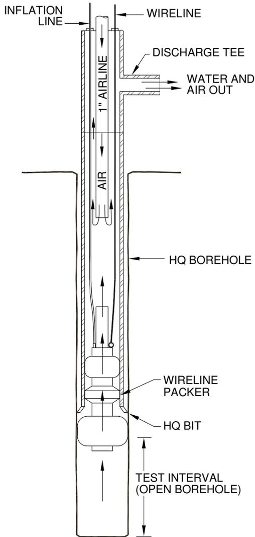
Figure 2. Setup for airlifting corehole with wireline packer assembly
