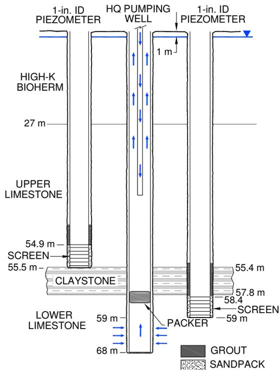
Figure 5. Testing  $K_v$  across a thin aquitard by airlift pumping in a packer-isolated HQ corehole
